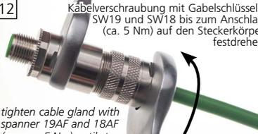
tighten cable gland with spanner 19AF and 18AF (approx. 5 Nm) until stop
