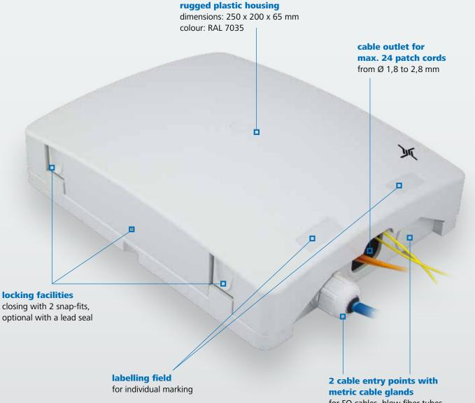
for FO cables, blow fiber tubes (from  $\emptyset$  5 to 9 mm) or TICNET cable-splitter ODS-Mini
